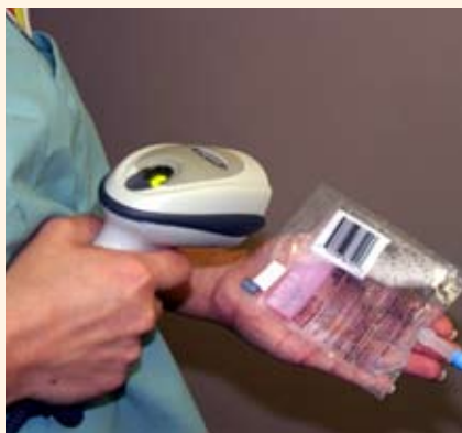
Before administering any medication, Union Hospital nurses use a handheld device to verify that the patient, medication and dose are correct.
